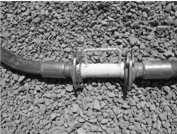
Figure 11. Coupling used for connecting lengths of pump hose and connecting pump hose to crane hoist cable.
