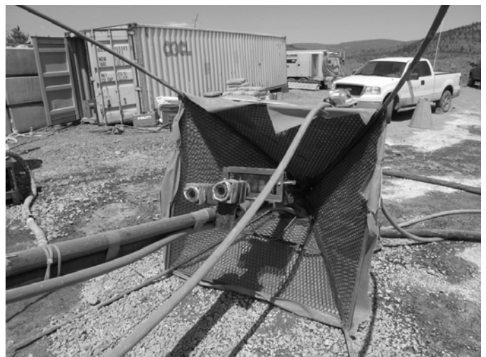
Figure 9. View of TV cameras mounted at top of “egg”.
